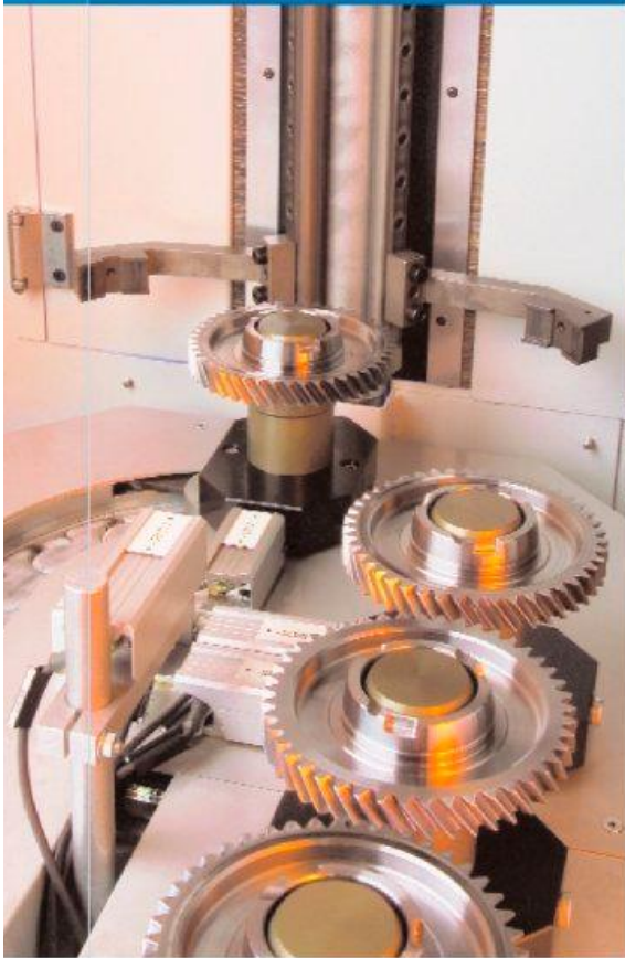
Genesis cam-driven double-gripper loader reduces load/unload time.
